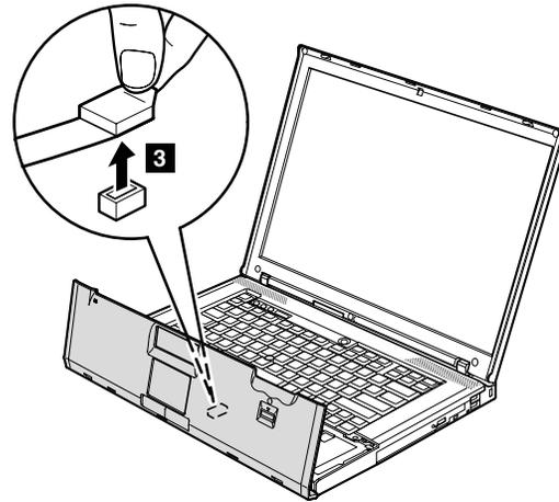
**When installing:** When you attach the palm rest, do as follows:
