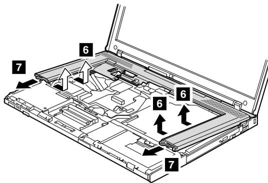
**When installing:** Make sure that all the claws are attached firmly.
