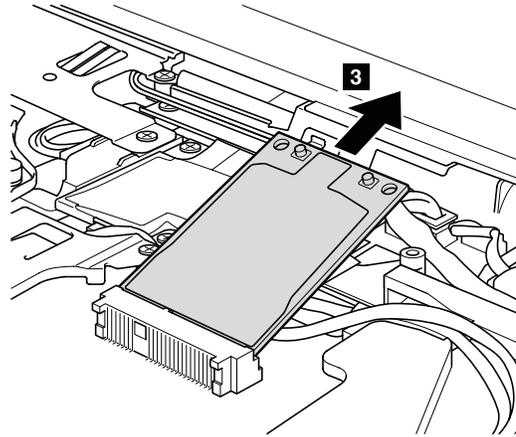
**When installing:** Plug the gray cable into the jack labeled **MAIN** on the card, and the black cable into the jack labeled **AUX**. If the computer you are servicing has three cables, put the white cable in the cable bag in the card slot
