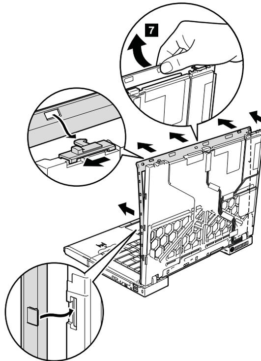
Table 35. Removal steps of LCD front bezel and LCD rear cover (LCD cover kit) (continued)
