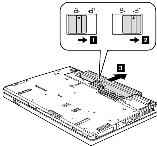
**When installing:** Install the battery pack along the slide rails of the slot. Then make sure that the battery release lever is in the locked position.
