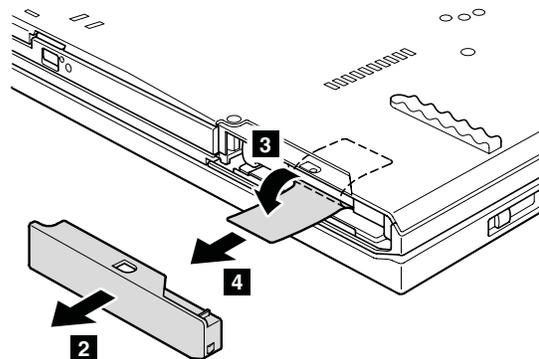
**When installing:** Make sure that the HDD connector or SSD connector is attached firmly.
