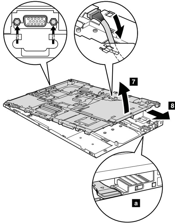
Remove the USB sub card with cable and the security hole bracket as in this figure.
