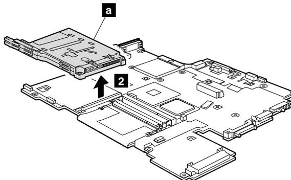
**When installing:** Make sure that the connector of the PC Card/Express Card slot assembly is attached to the system board firmly.
