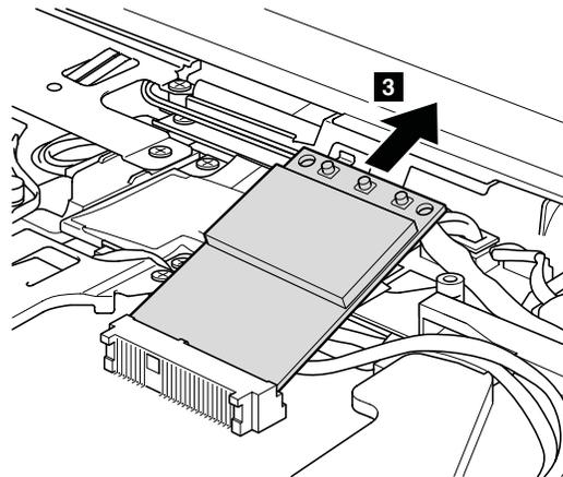
**When installing:** Plug the gray cable (MAIN) into the jack labeled TR1, the white cable (3rd) into jack labeled R0, and the black cable (AUX) into jack labeled TR2 on the card.
