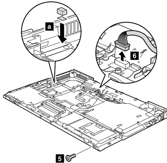
**For discrete graphics models:** When you are servicing, make sure that the thermal rubber for FET is firmly attached on the system board as shown in **a**. When replacing the rubber, you need to peel the thin film off from the bottom, and attach it to the system board.
