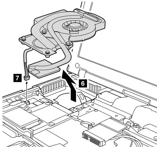
Table 28. Installation of the fan assembly
