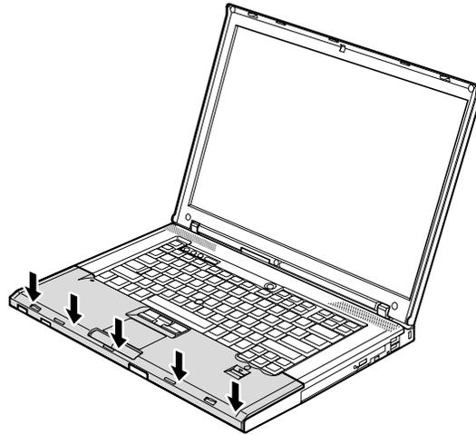
4. Close the LCD cover and turn the computer over. Then fasten the four screws to secure the palm rest.
