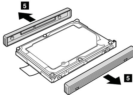
**When installing:** The rubber rails on the hard disk drive must be attached to the replacement drive. Otherwise the drive cannot be installed properly.
