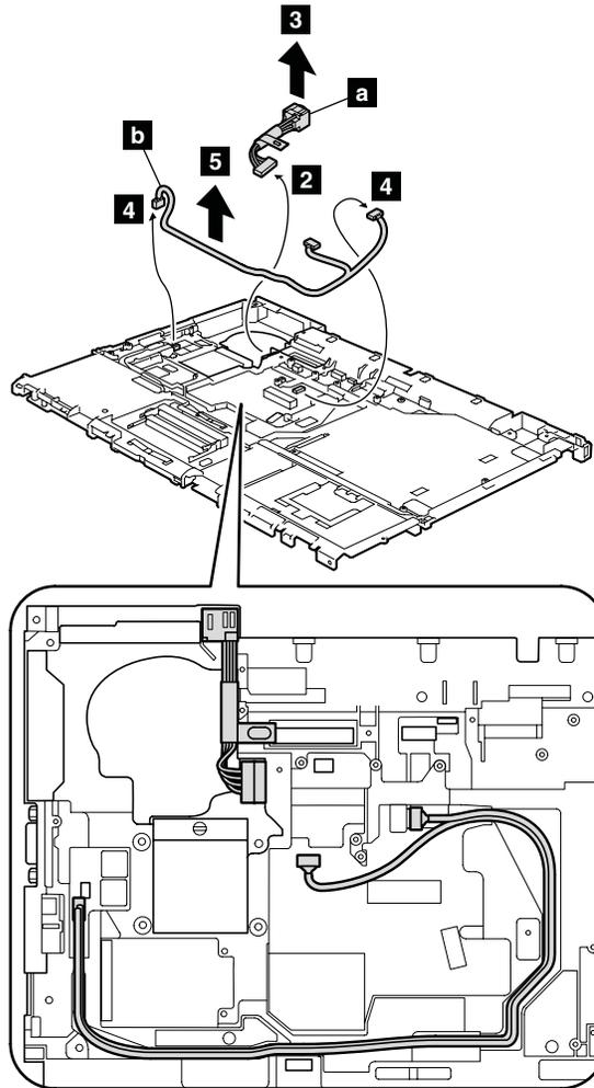
**When installing:** Make sure the connectors are attached firmly, and that the cables are routed as in the figure above.
