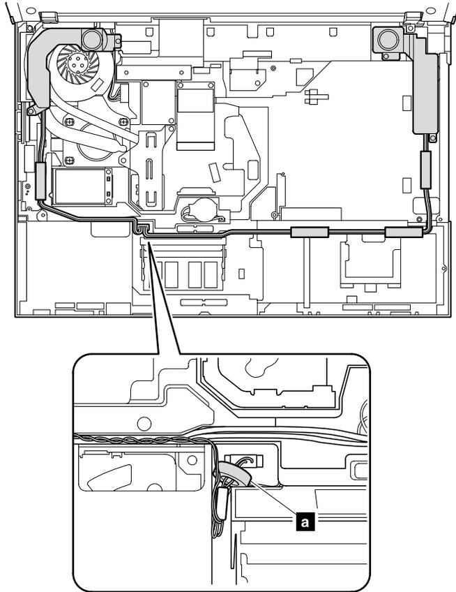
**When installing:** Make sure that the speaker connector is attached firmly, and the cables are routed as in this figure.
