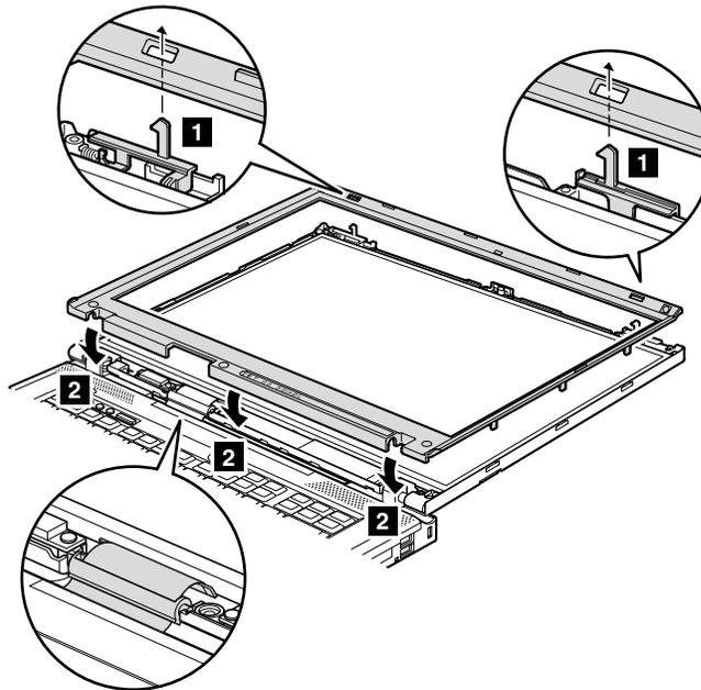
Table 36. Installation of the LCD front bezel and the LCD rear cover (LCD cover kit) (continued)
