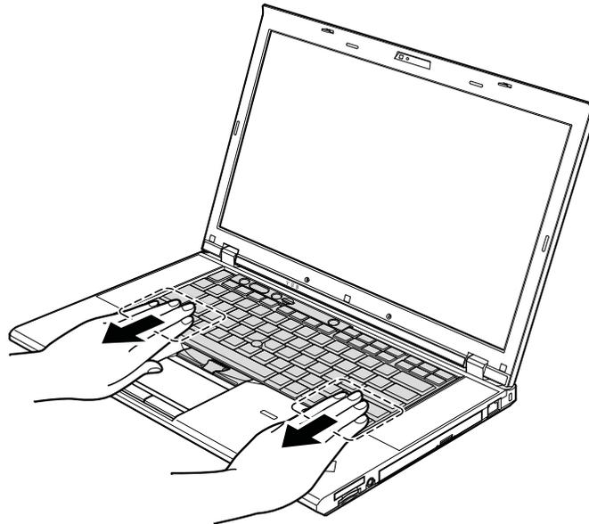
4. Make sure that the front side of the keyboard **b** is housed firmly.
