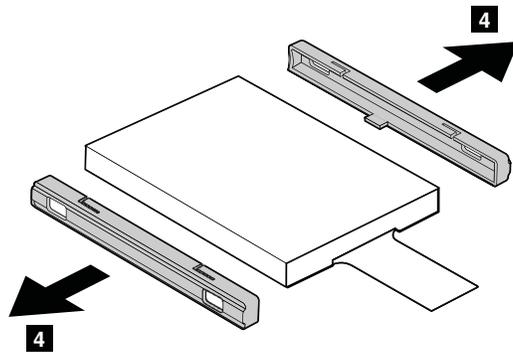
**When installing:** Make sure that the SSD connector or HDD connector is attached firmly.
