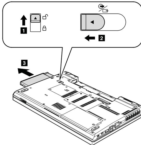
**Note:** For RAID models, the second hard disk drive adapter cannot be removed directly as shown in the above illustration until you remove the screw that secures the second hard disk drive adapter:
