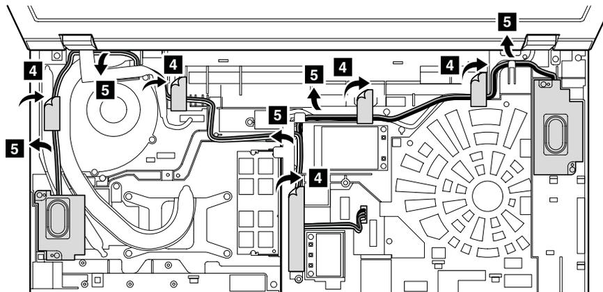
**When installing:** Make sure that the speaker connector is attached firmly. Then route the cables and secure them properly as shown in the figure above.
