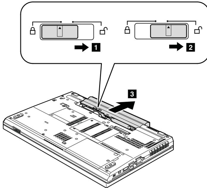
**When installing:** Install the battery pack in the slot, and then make sure that the battery latch is in the locked position.
