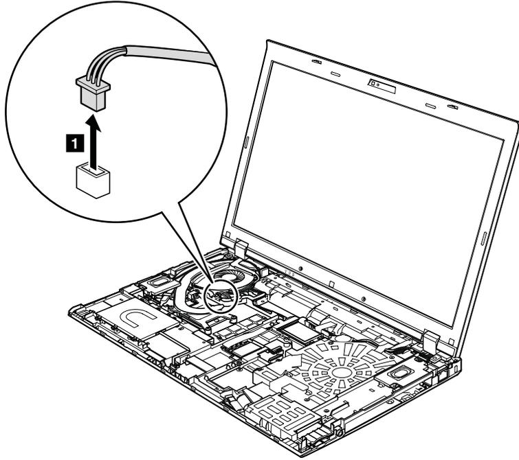
**When installing:** Make sure that the connectors are attached firmly.
