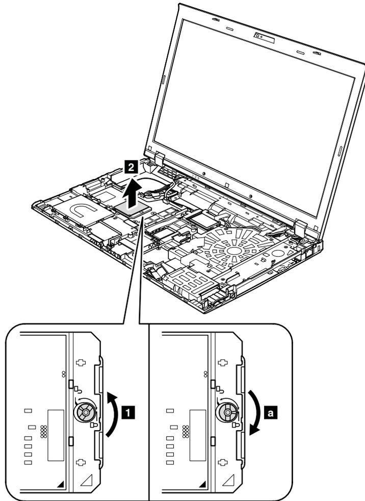
**When installing:** Place the CPU on the CPU socket, and then rotate the head of the screw in the direction shown by arrow **a** to secure the CPU.
