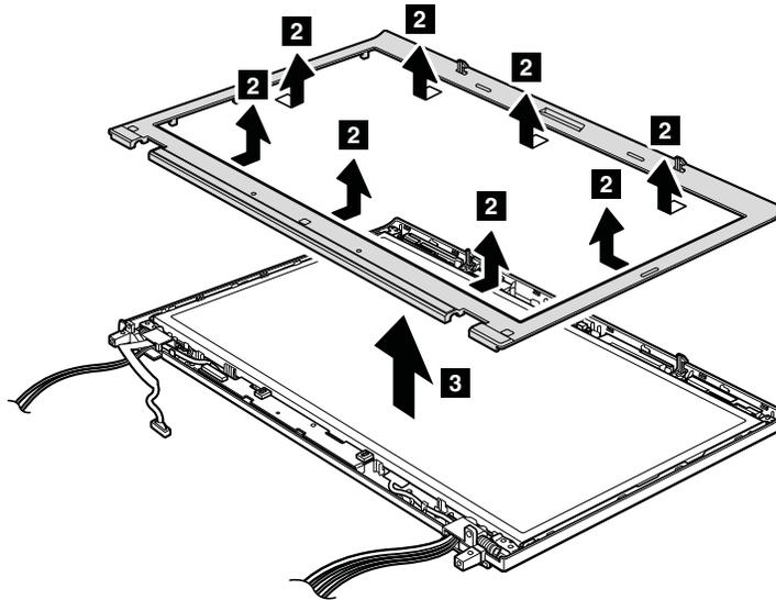
**When installing:** Make sure that all the latches are attached firmly.
