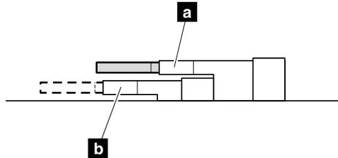
**When installing:** Insert the notched end of the DIMM into the socket. Press the DIMM firmly, and pivot it until it snaps into the place. Make sure that it is firmly fixed in the slot and does not move easily.
