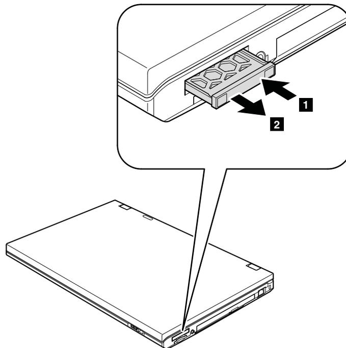
**When installing:** Make sure that the bezel or the card is correctly oriented as shown in this figure.
