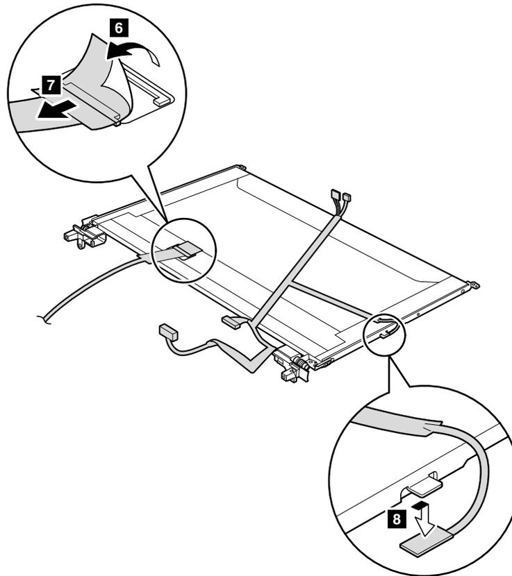
**When installing:** Make sure that the LCD cable connector is attached firmly.
