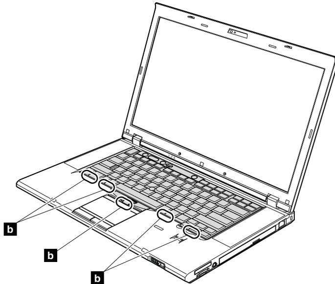
5. Secure the keyboard by tightening the screws from the bottom side of the computer.
