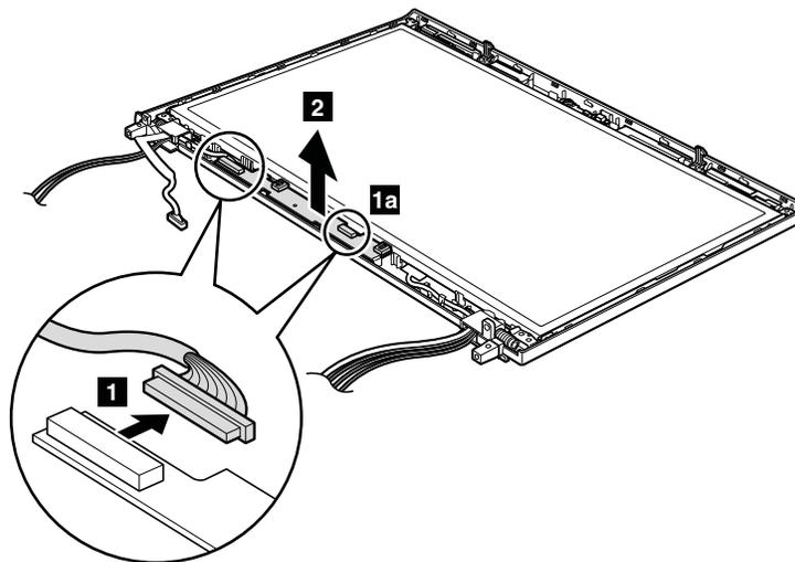
**When installing:** Make sure that the connectors are attached firmly and the card is installed as shown in this figure.
