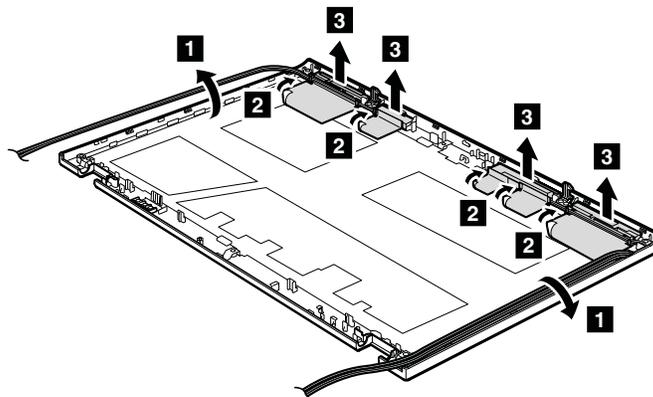
**Cable routing:** When you install the antenna kit, route the cables as shown in the figures below. As you route the cables, make sure that they are not subjected to any tension. Tension could cause the cables to be damaged by the cable guides, or a wire to be broken.
