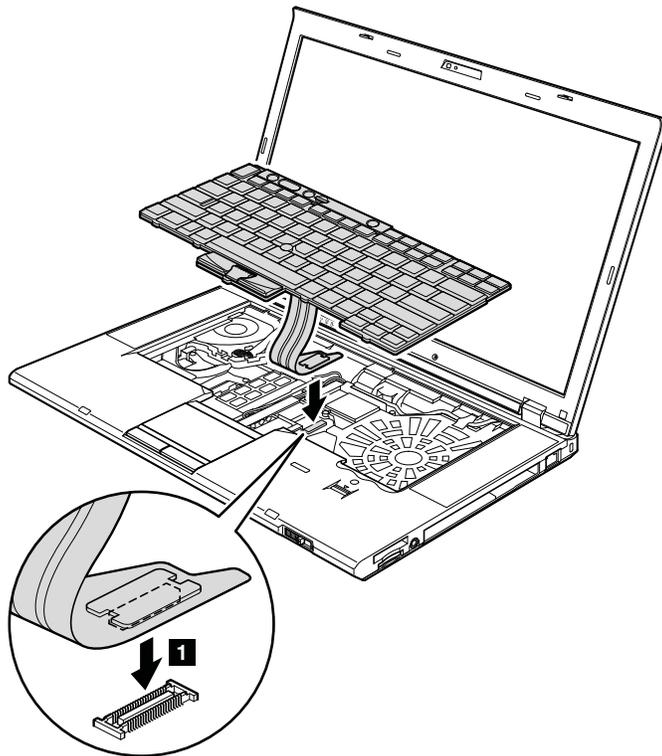
2. Attach the keyboard so that the keyboard edges **a** are under the frame as shown in this figure.
