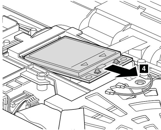
**When installing:** Plug the orange cable into the jack labeled **MAIN**, and the blue cable into the jack labeled **AUX** on the card.
