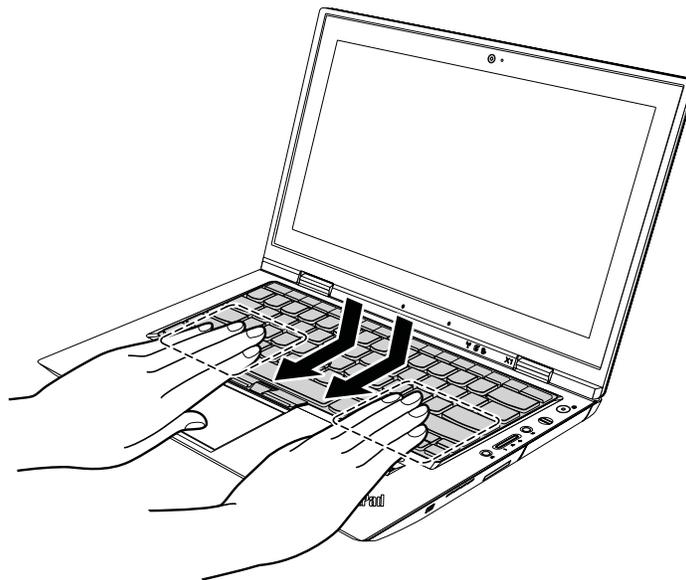
4. Make sure that the front edge of the keyboard **b** is attached firmly.
